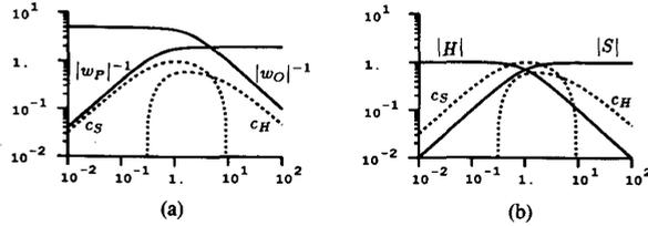
Fig. 3. Graphical representation of conditions (33) and (34). R.P. is guaranteed since  $|S| < c_s$  for  $\omega < 2$  and  $|H| < c_H$  for  $\omega > 1.4$ .
