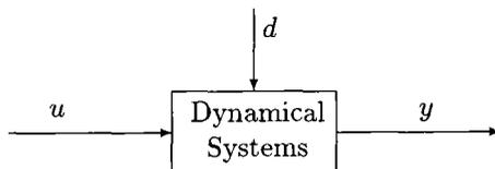
where  $u$  is the input sequence,  $y$  is the output sequence, and  $d$  is the disturbance in the dynamic
